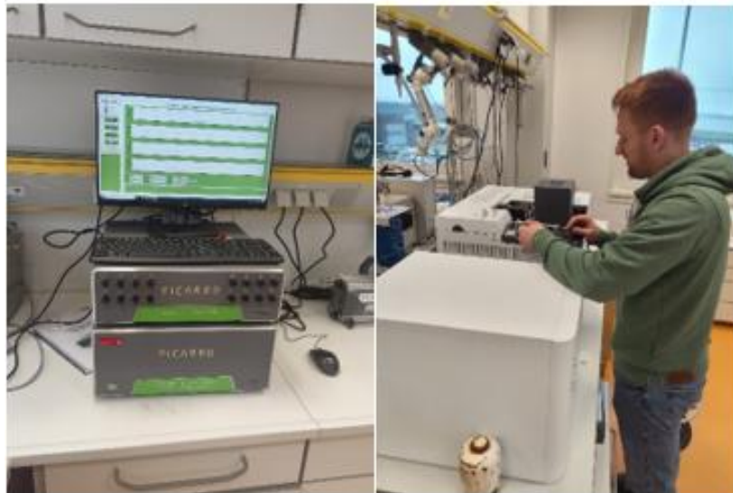
Figure 4. Ship-capable cavity ring down and gas chromatograph systems for the isotopic and compositional analysis of dissolved gas hydrocarbons.
